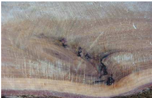
Figure 1. Overgrown branch with ingrown bark resulting in a major structural defect
