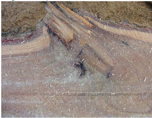
Figure 2. Branch stub with associated ingrown bark, this sometimes resulted in the development of doze that would travel into the centre of the log
