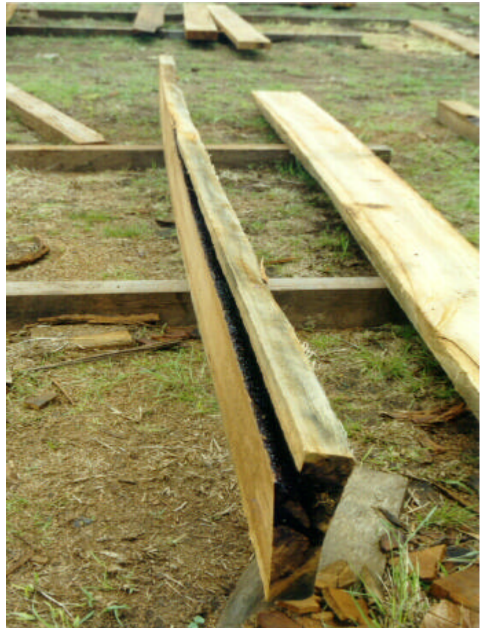
Figure 1 - Possible Tordon related stem defect
